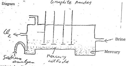
Concentrated sodium chloride (Brine) is the electrolyte The anodes are graphite. The cathode is the mercury
